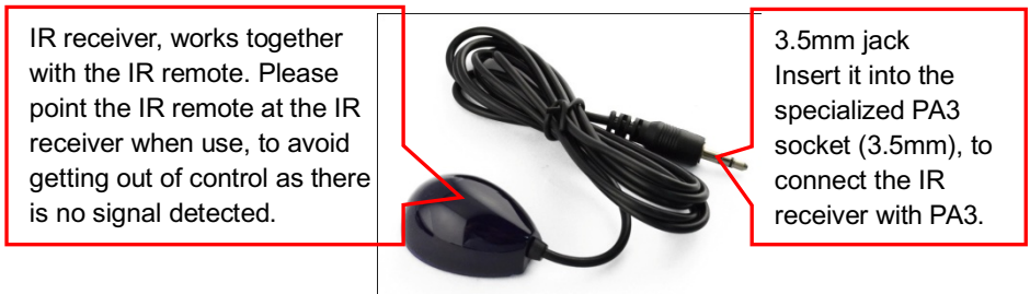
Figure 9 IR Receiver
